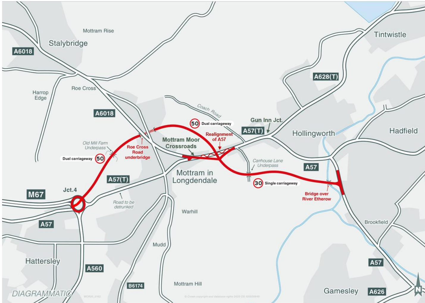
Figure 2-2 – A57 link road scheme alignment
